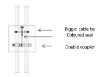
In this step, the EFL is put on two fences, so that each one remains vertical in the couplers. In case of only one fence to escape through, the EFL connects to the immovable fence.
