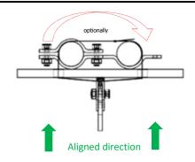
Please note the direction of the cutting edge in relation to the direction of the emergency escape direction. Be careful that both the fences can be opened. If only one opens, put the EFL at the immovable fence. If this rule is disregarded, a quick escape will not be possible.
